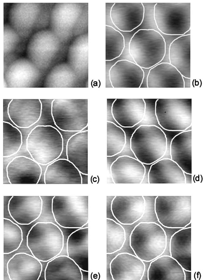
FIG. 5. Set of images (scan area  $1.5 \times 1.5 \mu\text{m}^2$ ) of the latex sphere test sample: topographic image (a), optical image obtained with polarization modulation (b), optical images for a fixed incoming polarization at  $0^\circ$  (c),  $45^\circ$  (d),  $90^\circ$  (e), and  $135^\circ$  (f).
