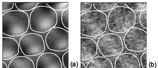
FIG. 4. Optical images (scan area  $1.5 \times 1.5 \mu\text{m}^2$ ) of the latex sphere test sample. The white lines reproduce the shape of the spheres obtained by the topographic image not shown. The two images have been acquired with an interval of a few minutes on the same sample area, but the results are quite different due to the different coupled polarizations.
